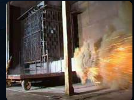
TPR6 HP - Internal Arc Proof Test 36kV - 25kA (CESI)
